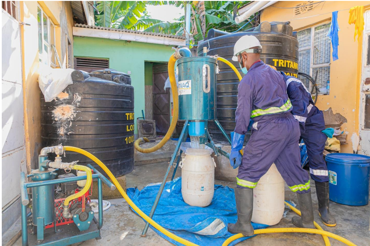
Photo: Arusha depot member in action, using Pit Vaq-an improved and semi-mechanised emptying equipment"
