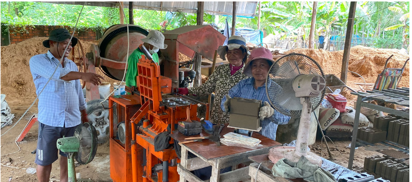
Since partnering with iDE in 2012, this latrine business in Kampong Thom province, Cambodia, has gone from strength to strength, including investment in an interlock brick machine to produce disability-inclusive toilet shelters Credit: iDE / Hang Seyha
