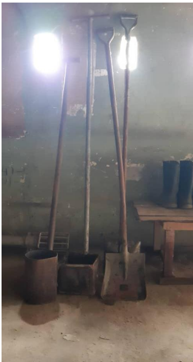
Figure 5: Scoopers and a modified shovel used to empty pits.
