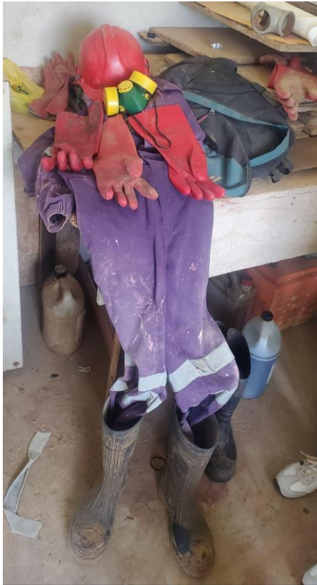
Figure 4: PPE for formal manual emptiers for one of the CU including gumboots, gloves, work suit, helmet and respirators.
