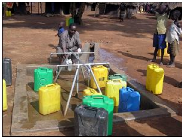
Plate 13: Water analyst (DWD) taking a sample from a motorised borehole with six outlets
