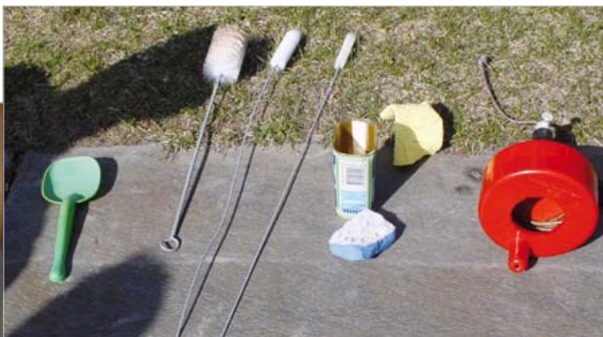
Figure 7: Cleansing tools for urine piping in a urine diverting toilet. Photo by Ebba af Petersens
