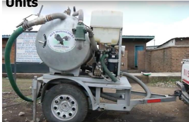
Mechanical De-sludging Units
